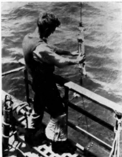
A string of Nansen bottles, such as this being lowered from the E. W. Scripps, of the Scripps Institution of Oceanography, is used to obtain samples of sea water at different depths.
